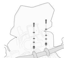
05SKITK Specific kit to mounting the KS900A Smart Bar
