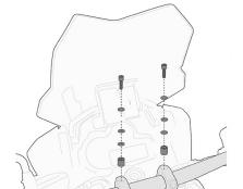
035KITK Specific kit to mounting the KS900A Smart Bar
