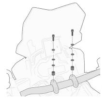
**015KITK** Specific kit to mounting the KS900A Smart Bar
