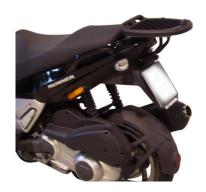
it is necessary to puncture the housing behind the saddle / maximum load allowed 3 Kg / to be combined with the plate already included in the MONOLOCK® top-case
