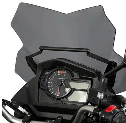
**KFB3112** Fairing upper bracket to be mounted behind the windshield to install KS920M, KS920L, KS95KIT and GPS-Smartphone holder
