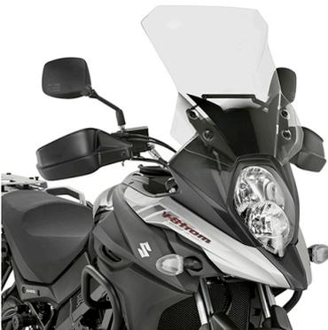
**KAF3112B** Specific sliding wind-screen transparent, Airstream. Maximum height 50 cm (12 cm of extension) width 43 cm
