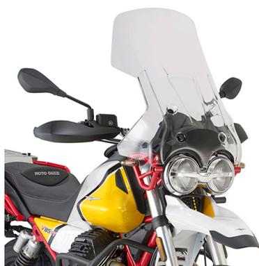
**KAF8203B** Specific sliding wind-screen transparent, Airflow. Maximum height 65 cm (12 cm of extension), width 50 cm
