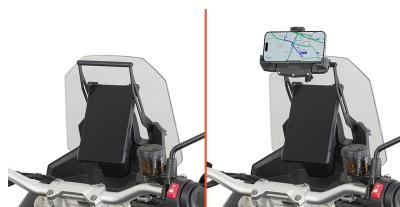
**KFB9651****Fairing upper bracket to be mounted behind the windshield to install KS920M, KS920L, KS95KIT and GPS-Smartphone holder**
