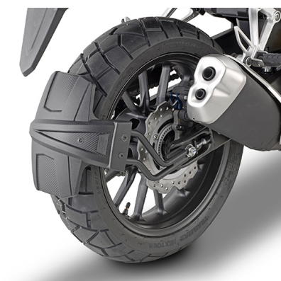
RM1171KITK Specific kit to install the spray guard KRM02
