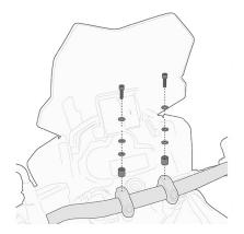
02SKITK Specific kit to mounting the KS900A Smart Bar
