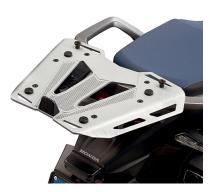
to be combined with the MONOKEY® KM5, KM7, KM8A, KM8B, KM9A or KM9B plate, or with the MONOLOCK® KM5M or KM6M plate / if combined with KM8A, KM8B, KM9A, KM9B it does not allow the assembly of the stop light kit or the remote control device on the case
