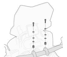
01SKITK Specific kit to mounting the KS900A Smart Bar
