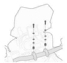
055KITK Specific kit to mounting the KS900A Smart Bar
