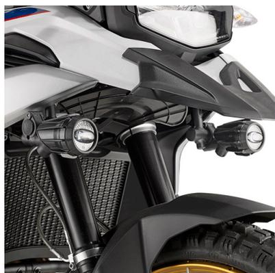
**LS5127K**    **Specific fitting kit to mount spotlights where specific engine guard is not present**
