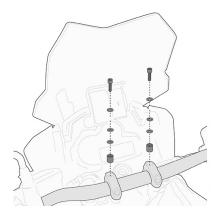
055KITK Specific kit to mounting the KS900A Smart Bar
