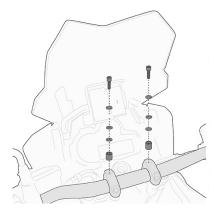
035KITK Specific kit to mounting the KS900A Smart Bar
