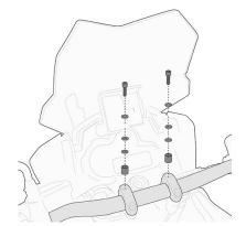
025KITK Specific kit to mounting the KS900A Smart Bar
