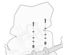
035KITK Specific kit to mounting the KS900A Smart Bar
