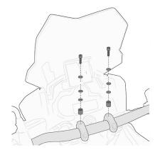
03SKITK Specific kit to mounting the KS900A Smart Bar
