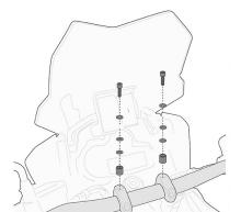
04SKITK Specific kit to mounting the KS900A Smart Bar
